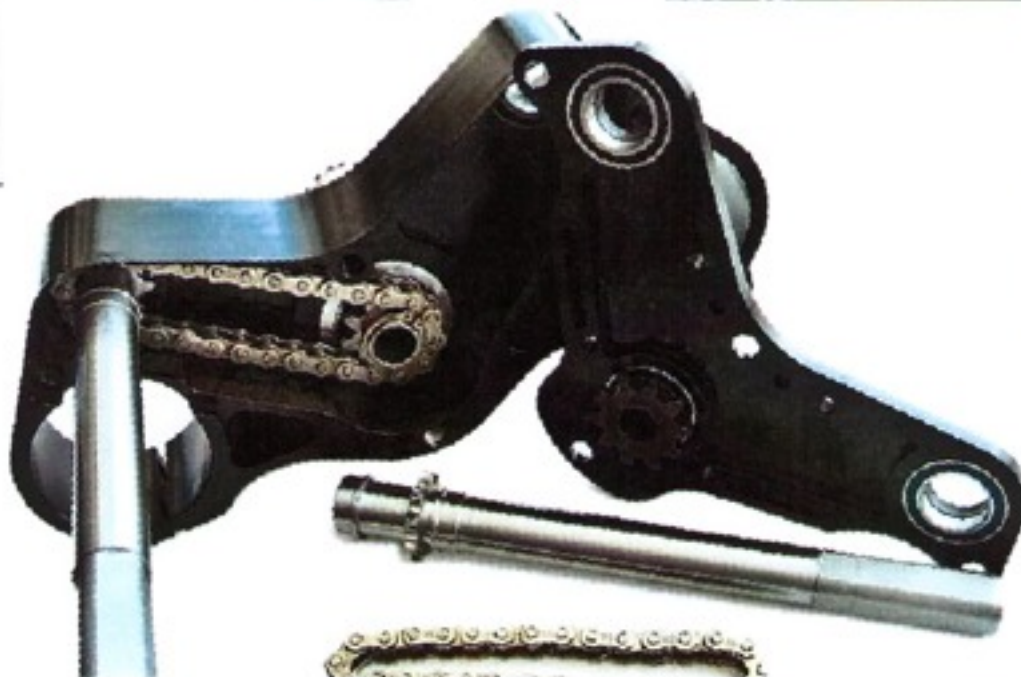
3D drawing illustrates the complexity of one of the components of the AWD system: the hub, whose two sprockets on the fork foot are fitted with helicoidal sprockets which are driven by the same number of spig cams which run along the fork rods. In the photos: the highly elaborate lower triple clamp sprockets and distribution chains, and the button on the handlebar to switch off integral traction when the bike is at a standstill.
