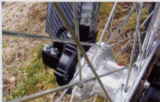
Up to 70% of the engines' power can be delivered via a system of chains, drive shafts and differentials to the enclosed chains that run from the modified steering head to the front hubs.
