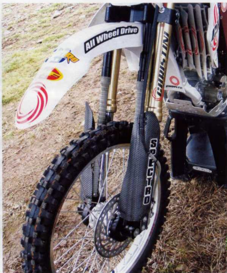
Up to 70% of the engines' power can be delivered via a system of chains, drive shafts and differentials to the enclosed chains that run from the modified steering head to the front hubs.
