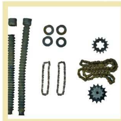
These were the parts we chose to replace after our tear-down. It was basically the second time for the chains.
