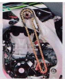
Thanks to EFI, there is more room to work with, and the KX450F is the narrowest feeling Christini we've ever ridden. Heavy frame modification is necessary to fit the gearbox.
