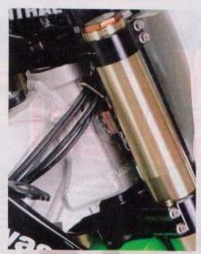
The two-wheel drive system requires a larger head tube and serious framework.
